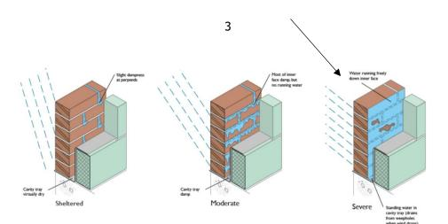
As there will be a cost of scaffold for investigatory works in any case, we would recommend that provision be made for cutting out and replacement of the cavity trays on all faces of the bay window so that new proprietary cavity trays with fixed stop-ends and interlocking corners can be installed, together with sufficient weep vents to let the water weep out.
